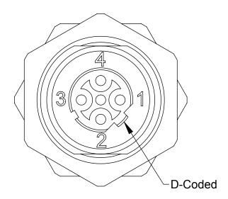
EtherCAT Connector 4 pin Female M12 D-Coded
